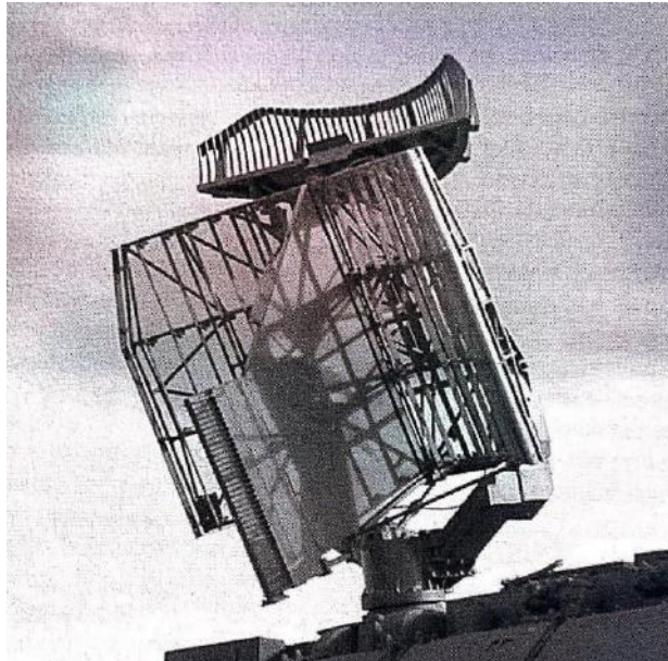
Figure 4-7. IFF antenna above the Target Acquisition Radar
